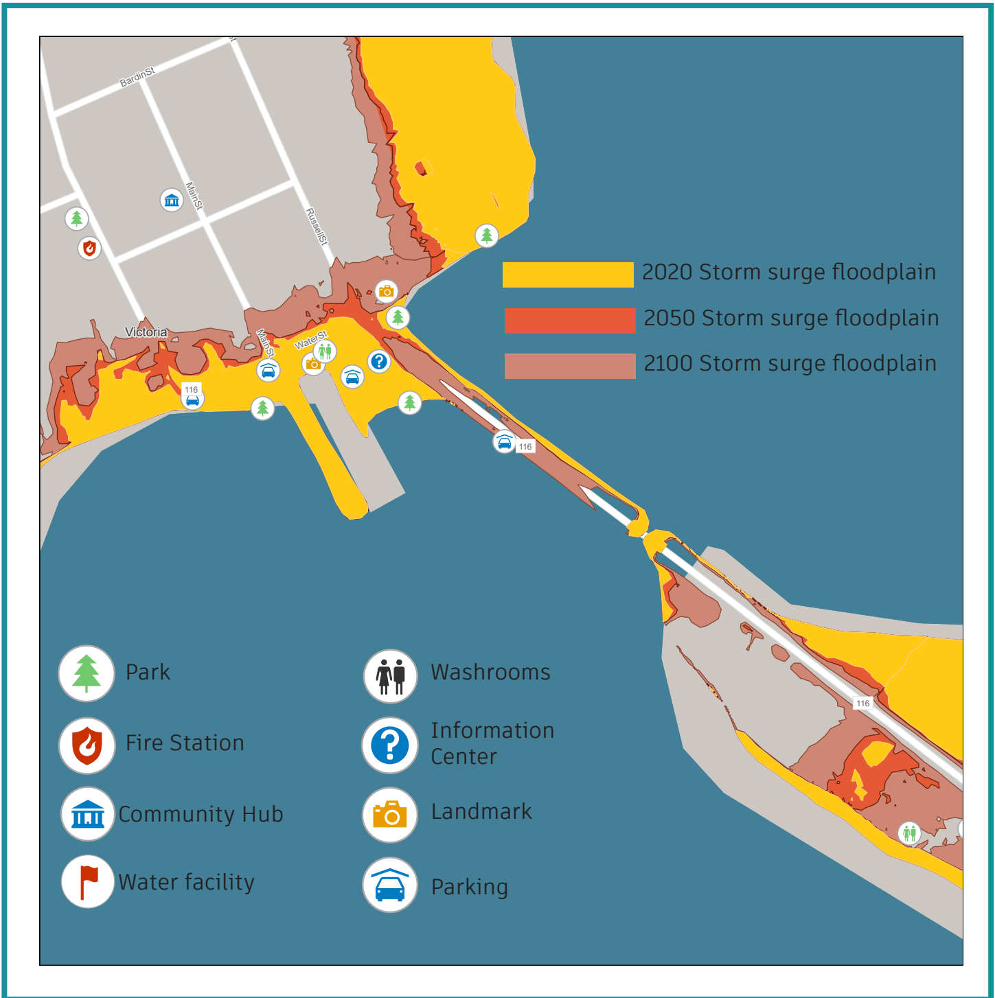
Figure 19: Post tropical storm and inland flooding impacts on municipal assets
